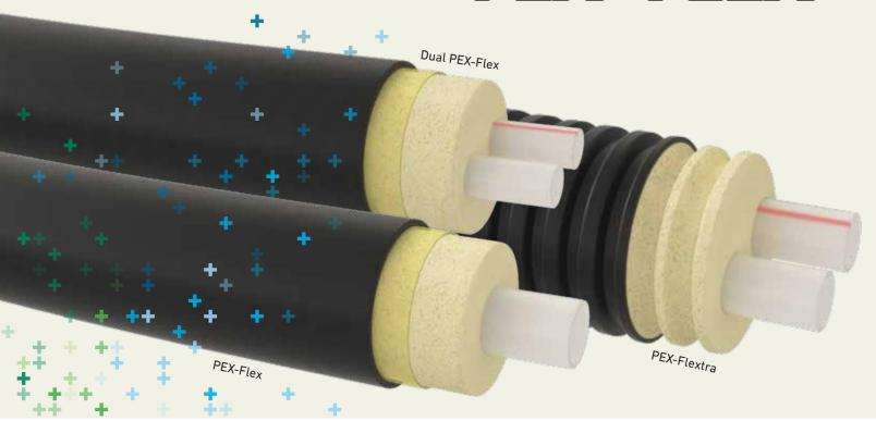
**PEX-Flex** is a pre-insulated pipe system complete with bonded polyurethane foam insulation and extruded polyethylene jacket. It is ideally suited for hydronic heating applications including campus style district energy, snow/ice melt systems and alternative fuel boilers such as outdoor wood furnaces. Supplied in coils and available with core PEX up to 4" single and 2" dual pipe, this seamless pipe system is economical, simple to install and highly effective even in harsh soil conditions.
